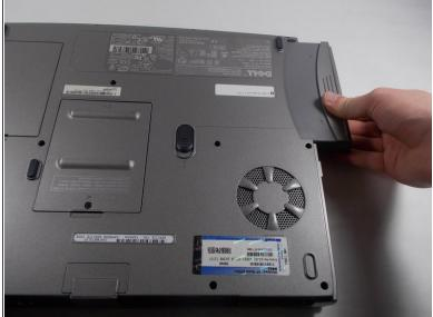
While holding the switch down, pull the battery out of the laptop, located in the upper right-hand corner.
