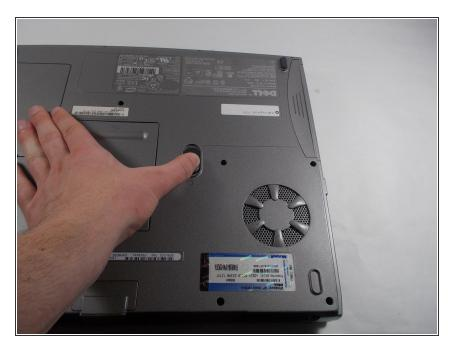
Locate the black switch on the back side of the device. Slide it to the unlocked position and hold it in place.
