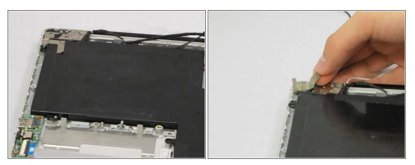
• Lift the strip tape away from the battery, being careful not to completely remove it.
