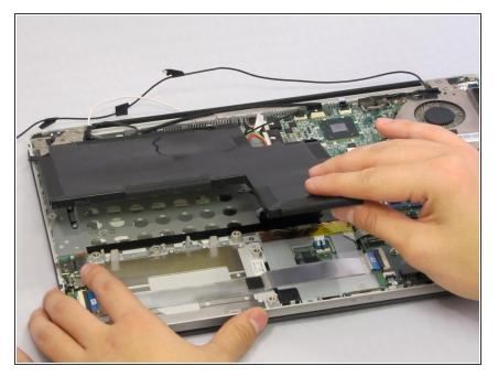
• Remove the battery by lifting up and away from device.
