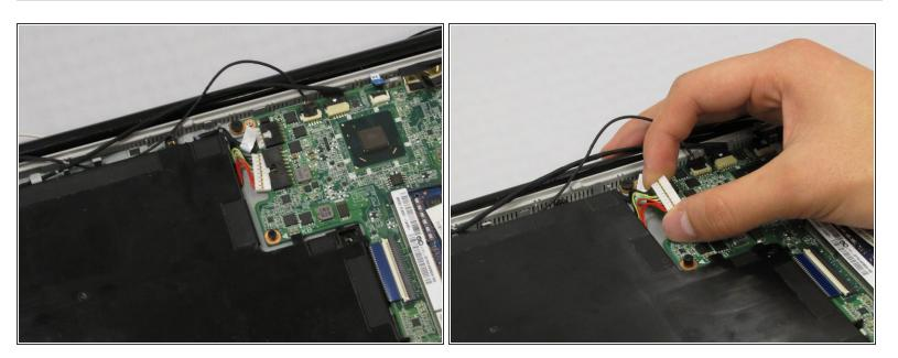
• Unplug the Battery from the circuit board by carefully prying the connector from its housing.
