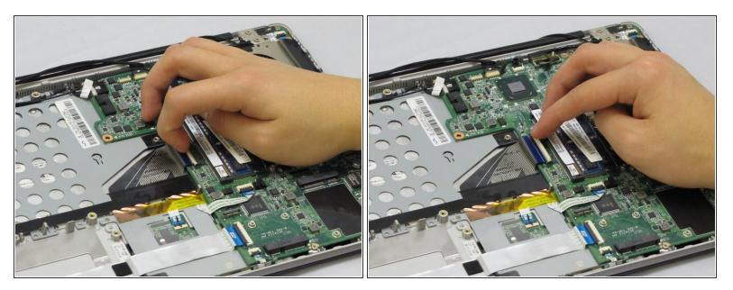
• Pry up the hinge that houses the keyboard's ribbon cable.
