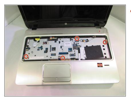
Using a Phillips #1, remove the four 5.6mm silver screws.
