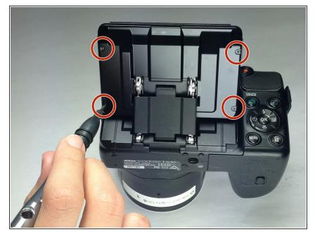
Use a Phillips head P000 screwdriver to remove the four 3.0 mm Phillips screws on the back of the monitor.
