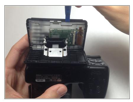
Use a plastic opening tool to remove the front cover of the LCD monitor, allowing the monitor to be completely be released.
