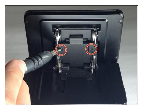
Use a Phillips head P000 screwdriver to remove the two 3.0 mm Phillips screws on the hinge cover.
