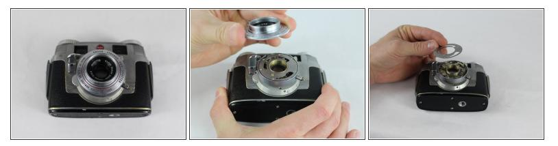
• While the camera is lying on its back, unscrew the front lens assembly and remove the lens and the faceplate. Then lift off the speed setting.
