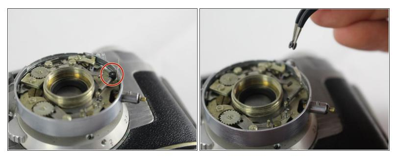
• Remove the stopper by lifting it upwards with the tweezers.
