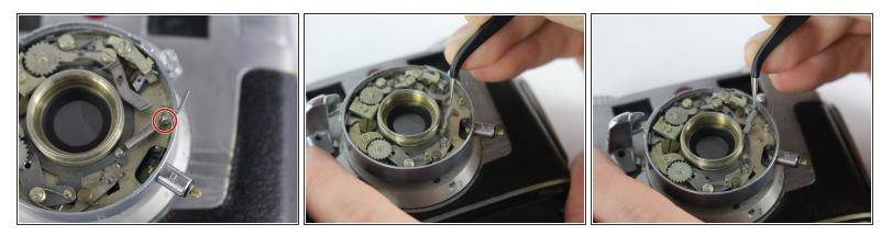
• Using tweezers, unhitch the spring from the base and remove it by lifting upwards.
