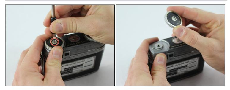
• While holding the rewind dial with one hand, remove the 2.8mm flathead screw that holds it in place with the 2.5mm flathead screwdriver.
