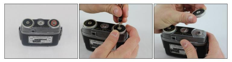
• While holding the wind dial with one hand, remove the <u>2.8mm flathead</u> screw that holds it in place with the 2.5mm flathead screwdriver.
