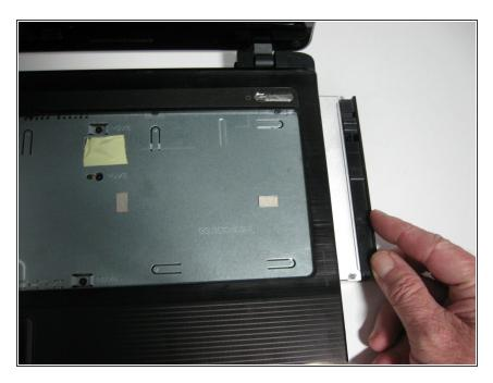
Remove the optical drive from the laptop by pulling it to the right until it has been fully detached from your laptop.
