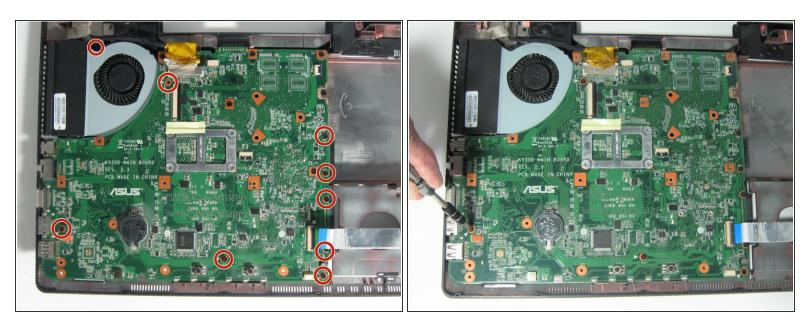
Remove nine 7.0 mm Phillips #0 screws from the motherboard using your Phillips #0 screwdriver.
