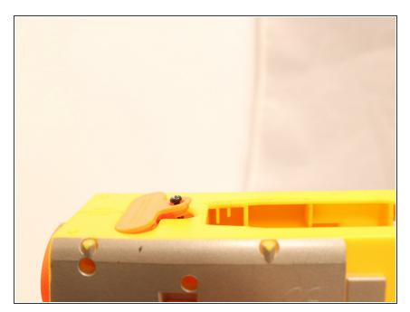
• The lid that covers the batteries should then rise up slightly, allowing it to be pulled off.
