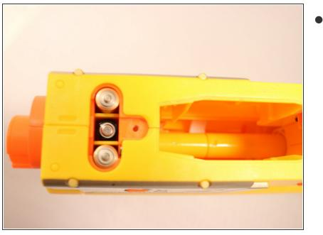
• Remove the batteries.
