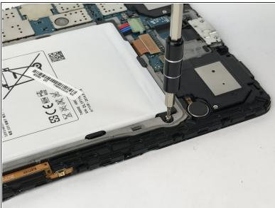
Remove the four 2.5mm Phillips #000 screws.
