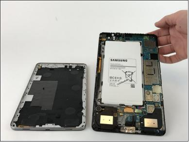
• Continue around the entire device until the back panel is completely separated from the screen.
