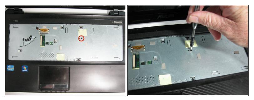
• Remove the single silver 6.0 mm Phillips #0 screw that connects the optical drive to the palm rest.
