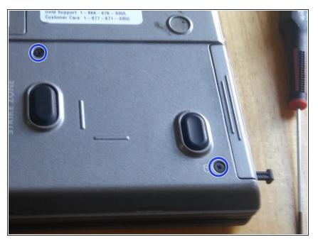
Now, remove the two drive screws, located in the bottom right of the laptop. These are helpfully labeled with a cylindrical hard drive icon.
