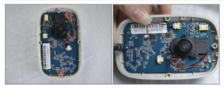
• Use a Phillips #0 screwdriver to take out the two 1.2 mm screws on the board.
