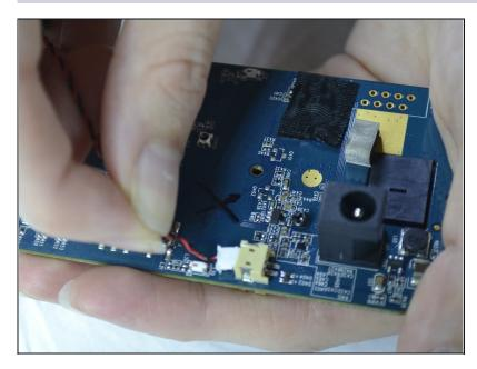
• The speaker wires are attached with the board. It can be unattached gently by pulling out the white attachment from the port.
