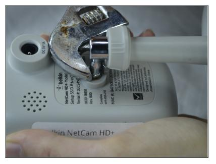
• Use a wrench to loosen up the stand from the back in order to hold the NetCam more comfortably.
