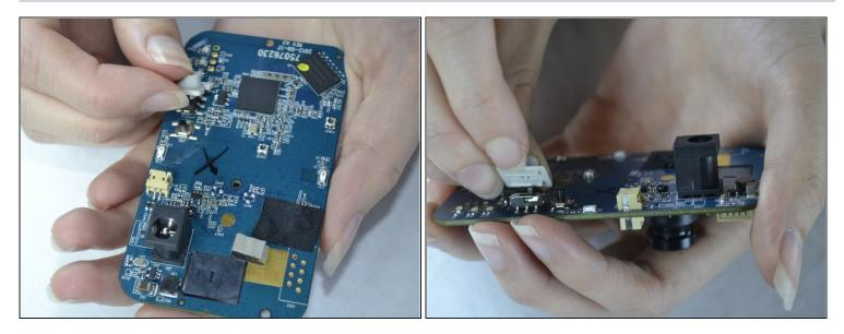
• On the back of the board pull the switch slowly upward to take it off.
