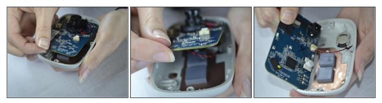
• With your fingers, pull the circuit board out of the back casing.
