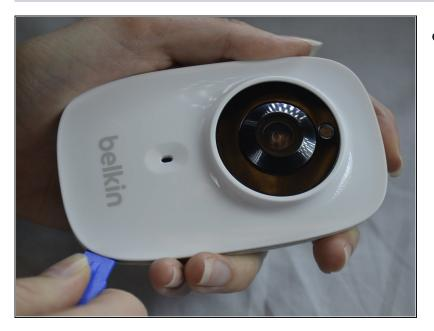
• Work a plastic opening tool into the seam and pry the face plate away from the back panel.
