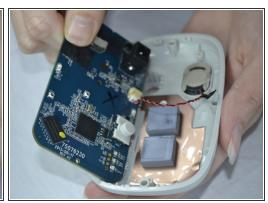
With your fingers, pull the circuit board out of the back casing.
