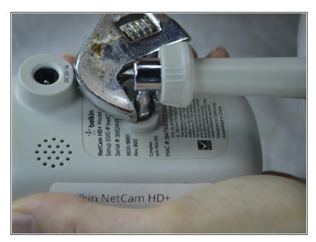
Use a wrench to loosen up the stand from the back in order to hold the NetCam more comfortably.
