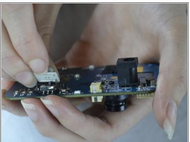
On the back of the board pull the switch slowly upward to take it off.
