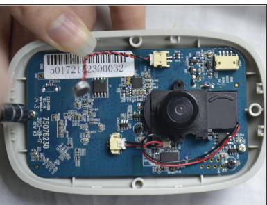
Use a Phillips #0 screwdriver to take out the two 1.2 mm screws on the board.
