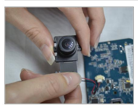
Slide the attached piece from the lens holder device.
