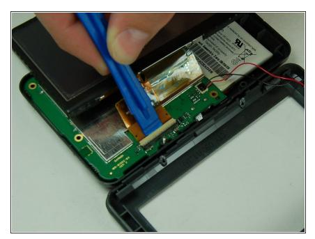
Use a plastic opening tool to gently lift up the white rectangular snap clip that is attached to the screen.
