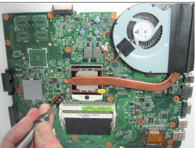
Remove the four 6.0 mm Phillips #0 screws from the heat sink using your Phillips #0 screwdriver.
