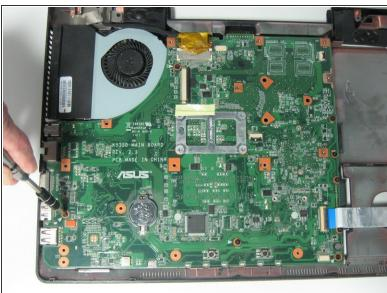
• Remove nine 7.0 mm Phillips #0 screws from the motherboard using your Phillips #0 screwdriver.
