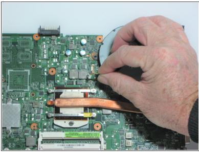
Disconnect the black, red, yellow, and blue set of wires from the motherboard using your fingers.
