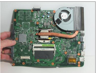
Turn the motherboard over to access the fan and the heat sink.
