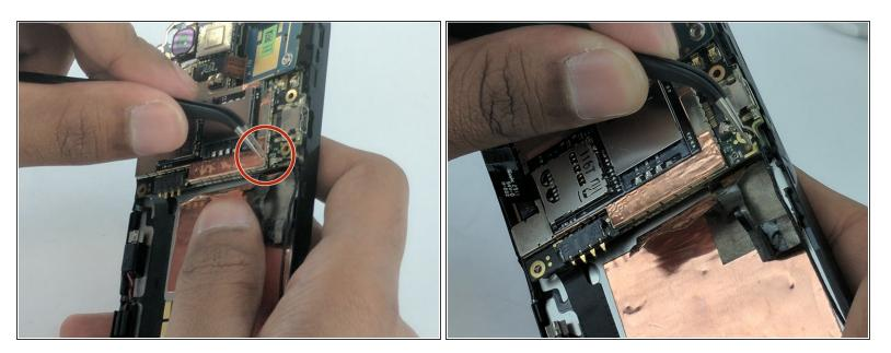
Remove the power supply from the motherboard by gently pulling the end of the black wire with the precision tweezers.
