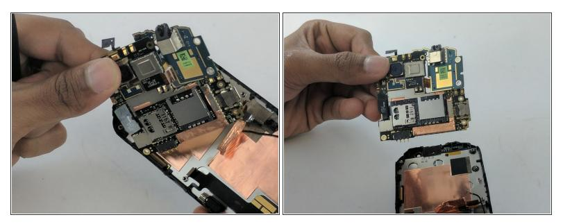
• Carefully pull the motherboard out of its recess.
