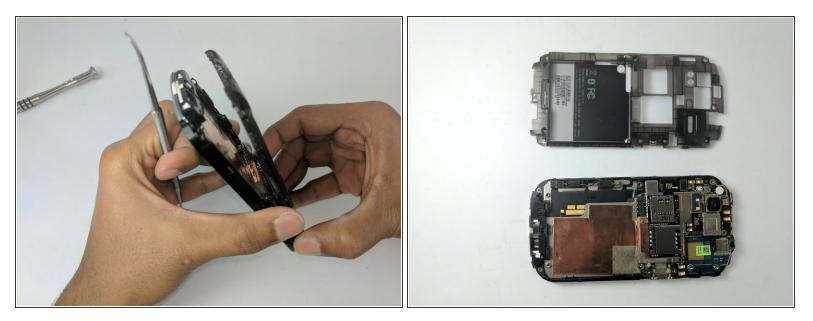
• Now simply remove the back panel by gently pulling. This will make it easier to access the devices internal components.
