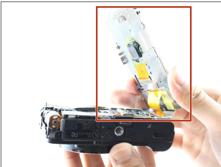
**⚠** LCD screen is very fragile. Handle with care. Do not use tools to remove the screen.
