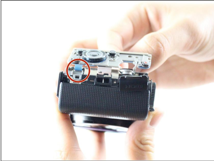
**⚠** Disconnect the control board data cable with care. Permanent damage may occur to the control board if tools are used to disconnect the data cable. Use your fingers only.
