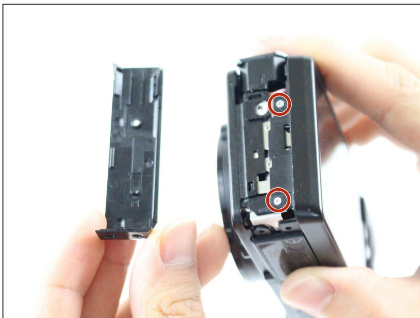
**⚠** The marked screws will loosen the rear case and the LCD screen may shift. The use of a soft work surface will prevent the LCD screen from breaking if it accidentally shifts during the removal process.
