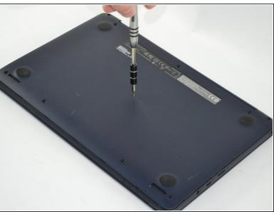
Unscrew all ten 2mm screws located on the bottom of the laptop using a Phillips #2 screwdriver.
