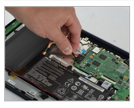
Disconnect the battery from the motherboard by pulling the No-Fuss Ribbon cables out of the connector.
