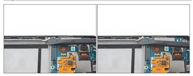
• Use the flat end of a spudger to disconnect the left antenna cable.
