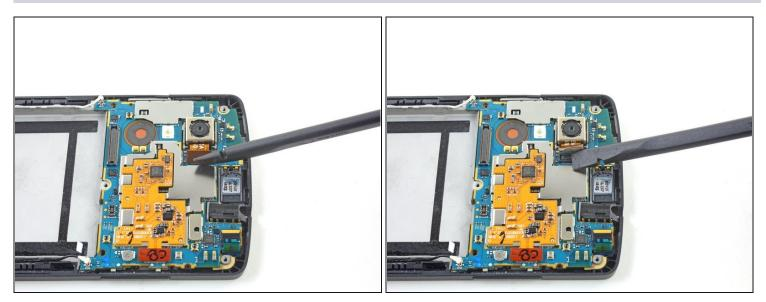
• Use the flat end of a spudger to disconnect the ribbon cable that connects rear-facing camera to the motherboard.
