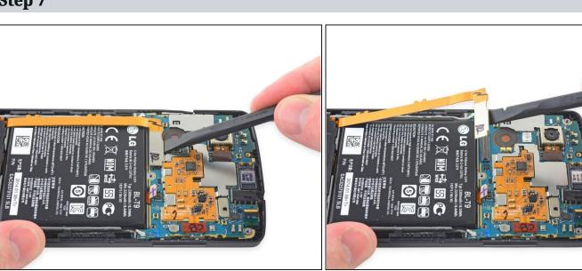
• Use the flat end of a spudger to disconnect the daughterboard ribbon cable and pull it away from the battery.
