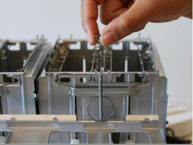
Remove the spring wrapped around a metal rod at the front of the toaster, located behind the white plastic lever holder.
