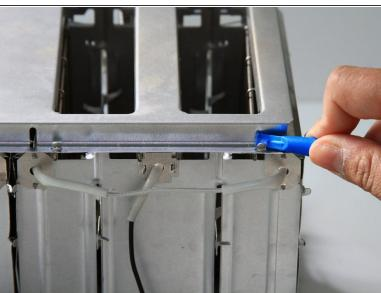
Use the plastic opening tool to remove the top metal panel by prying the 4 top metal tabs upwards.
