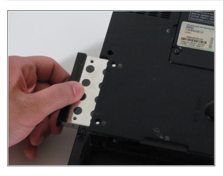
Slide the hard drive cage out from the hard drive compartment.
