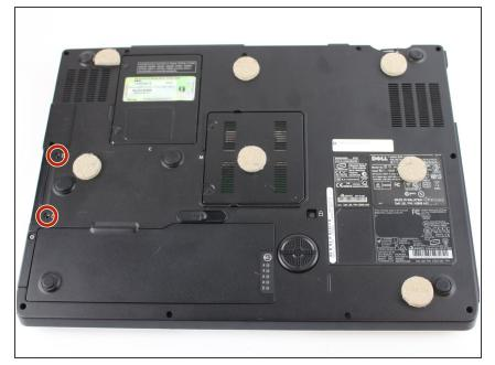
Remove the two 3mm Phillips screws.
