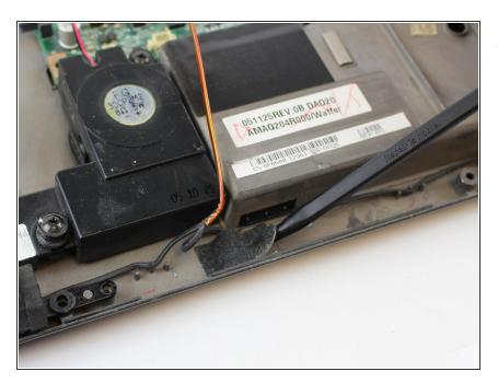
Pry away the black tape that holds the sound system wires in place.
