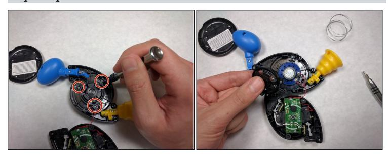
• Remove the (3) #3 Phillips head 6 mm screws using your Phillips #0 screwdriver, and remove the plastic with your fingers.
