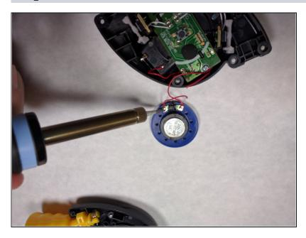
De-solder the speaker from the wires. Refer to the <u>soldering</u> guide for instructions on how to solder
