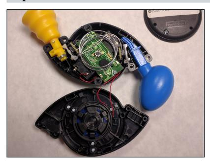
Carefully separate the two sections, leaving them connected by the wires.
