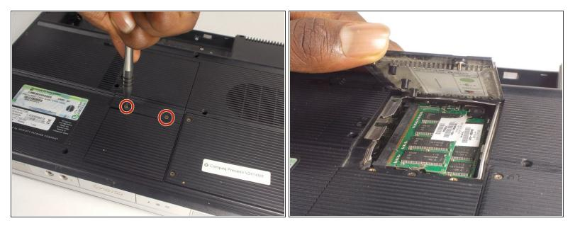
Loosen the two 5mm Phillips #1 screws that secure the memory module compartment cover to the computer.
