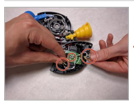
Remove the buttons by de-soldering them from the wires they are attached to or from the mother
