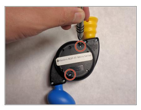
Loosen the two captive 8 mm screws in the back cover using a Phillips #0 screwdriver.
