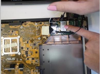
• Unscrew the two 3mm Phillips screws using a J1 screwdriver to release the Wi-Fi chip.
