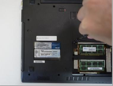
• Unscrew six 3mm Phillips screws in the RAM and hard drive compartment with the J1 screwdriver.
