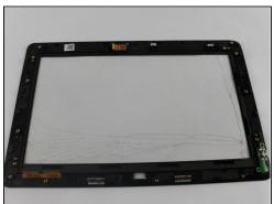
• Carefully use tweezers to lift the LCD screen from the digitizer touch screen.
