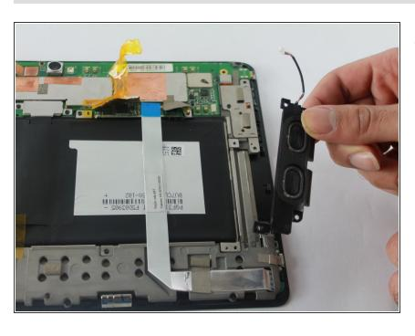
Remove the speaker from the device by lifting up on it. To reassemble your device, follow these instructions in reverse order.
