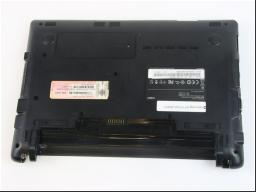
• Using your index fingers, push the battery outward, toward your body. The angle is somewhat awkward, but don't be afraid to use a little force. The battery should slide out in one motion.
