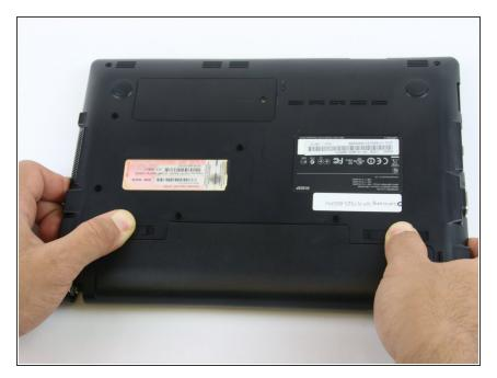
With both thumbs, slide the switches outward, away from the center of the laptop.
