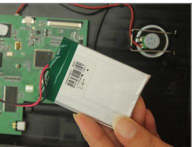
Remove the battery from the case by sliding a halberd spudger below it. (note: the spudger shown is metal, to ensure proper safety, utilize a nylon or plastic spudger.)
