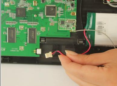
Disconnect the head of the cable attached to the motherboard by pressing on the outer edge of the cable and sliding it out.
