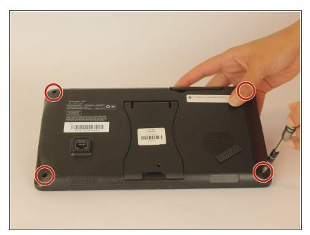
First, remove four 6.1 mm screws from your monitor using a J1 Phillips head screwdriver.
