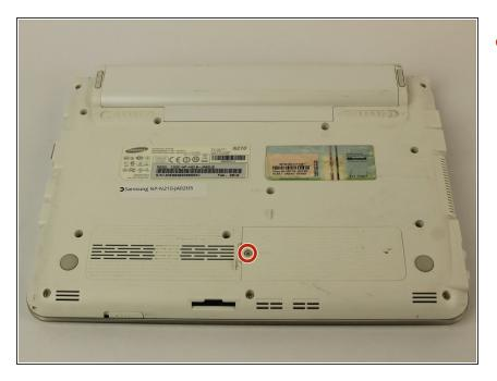
Remove the one 3.5 mm Philips #00 screw.
