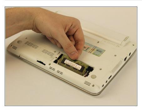
• Pull the RAM out of its socket.
