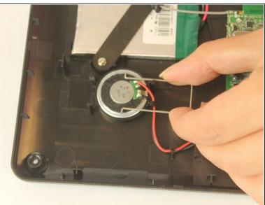
Locate the circular speaker in one of the corners of the device. To release the speaker, pinch the metal fastener together and lift it off of the speaker.
