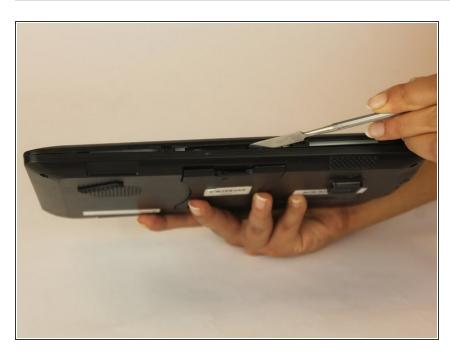
Using a metal spudger, open the monitor from the corner. Slowly slide the spudger around the case to prop open the case.
