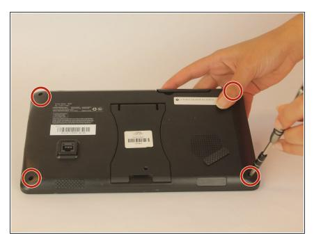
Using a J1 Philips head screwdriver, unscrew all four 6.1 mm screws.
