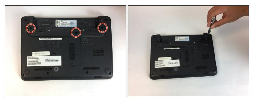
Unscrew three black 1mm screws using the PH1 Phillips-head screwdriver on the bottom of the laptop around the battery.
