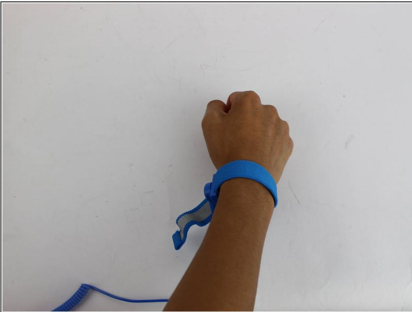
**⚠** Put on the anti-static wrist trap and clip it to a large metal object.
