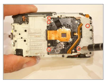
Using a Philips 000 screwdriver, remove the 5-(2.7mm long) screws from the silver plate that the lens is mounted to on the back (screen side) of the camera.
