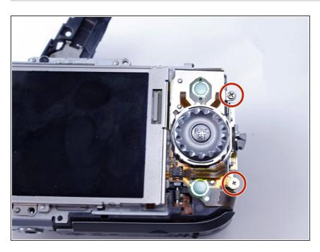
Remove two 3.2mm PH000 screws on the side of the camera, to the right of the button that reads "Func. Set."
