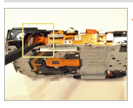
From the top of the camera, detach the flash assembly ribbon behind the flash bulb using the point of the spudger or small tweezers.
