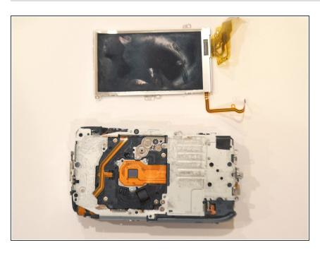
The LCD screen should now be removed from the body of the camera.
