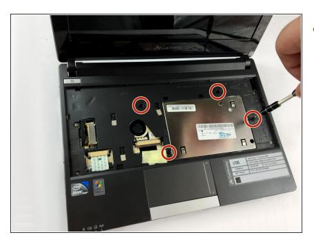
Using a Phillips #0 screwdriver, remove the four 6mm screws that secure the back access panel.
