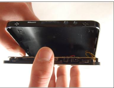
Use the plastic opening tool to pull the screen away from the back cover.
