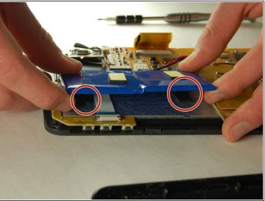
Once you have seperated the back plate and the screen from each other like so, you will then begin to lift the battery peeling it off of its sticky pads.
