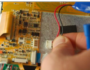
Unplug the battery at the plug indicated by the plastic opening tool. (The best way to do this is to place a finger on both sides of the plug and pull out gently) Once you have removed the old battery, plug the new battery into the same plug the old one came from.
