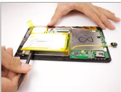
Use a spudger to pry the battery and detach it from the glue underneath it.
