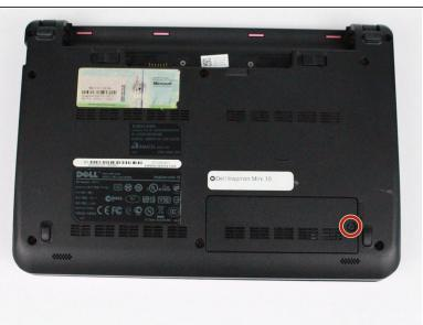
On the bottom of the laptop locate the removable panel and screw holding it to the body. Loosen the screw and take the cover off.
