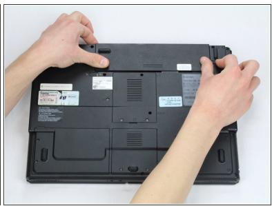
Pull the sliding switch to the right and continue to hold it in this position.
