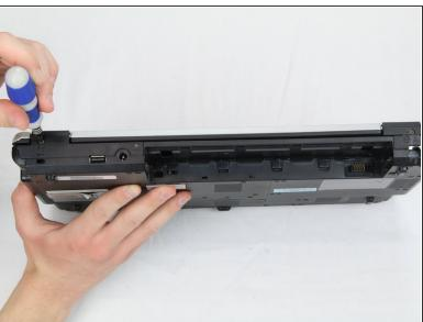
Remove the two circled 4mm screws with a J1 screwdriver.
