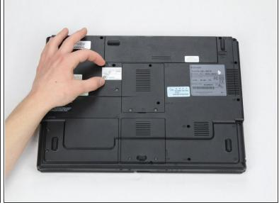
Slide the battery lock switch to the left.
