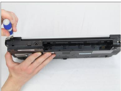
Remove the two circled 4mm screws with a J1 screwdriver.
