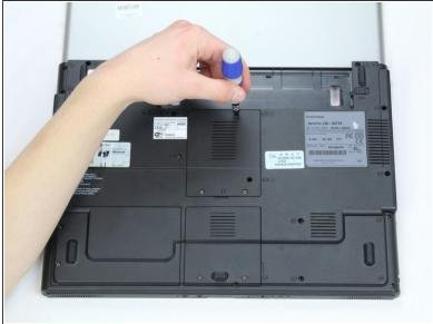
Remove the two circled 5mm screws with a J1 screwdriver.
