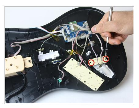
Using a size J1 philips head screwdriver, remove the two black 5 mm screws (circled in red) from the
