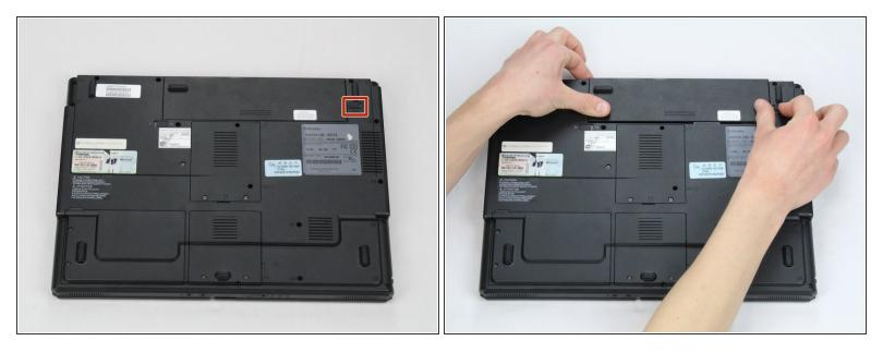
Pull the sliding switch to the right and continue to hold it in this position.
