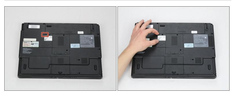
Slide the battery lock switch to the left.
