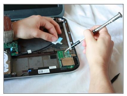
Use a J0 Bit screwdriver to remove the two 6 mm Phillips head screw located on the daughter board.
