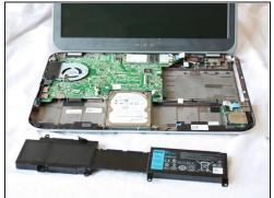
• Lift the tiny black tab and pull the battery out at a slight angle.
