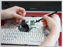
• Flip the little black securing bar near the base of the ribbon with a spudger to release the ribbon from the computer.
