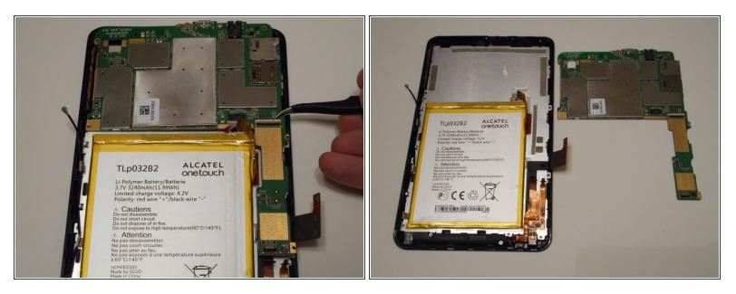
• With the screws removed, you can now remove the motherboard. Using tweezers or just your fingers, pick up the motherboard and place it to the side.
