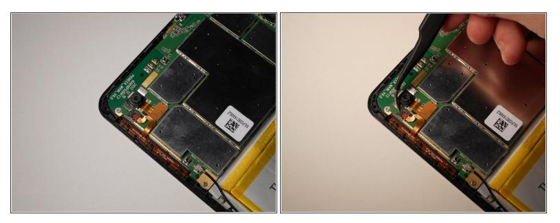
• The volume button assembly is in the top left corner of the tablet. To begin, you will have to pull the small black tab of the ZIF connector, shown in the second picture, to be able to remove the assembly. The tab is on a hinge so it should not be pulled off completely.
