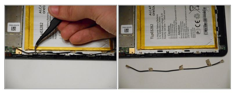
• With each of the antenna ends disconnected, you can pull out the full antenna. There will be 3 pieces of tape wrapped around the antenna and stuck beneath the battery. They may be a bit difficult to remove but not impossible.
