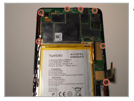
Using a PH00 screwdriver to remove these seven 2mm screws and place them in a safe spot where you won't lose them.
