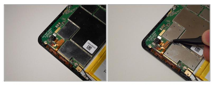
• The camera is in the top left corner of the tablet. To begin removal, use the tweezers to gently disconnect the ribbon cable attached to the camera.
