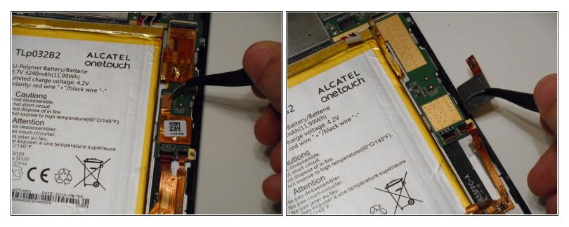
• Disconnect the ribbon cable and move it out of the way of the motherboard.
