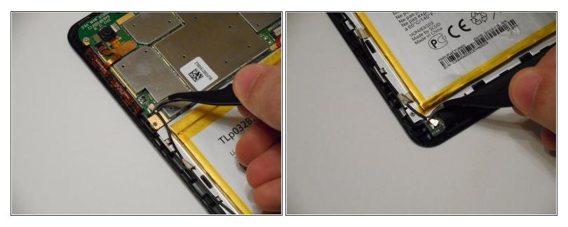
• Using the tweezers, pull the WIFI Antenna away from the motherboard and the wireless card.
