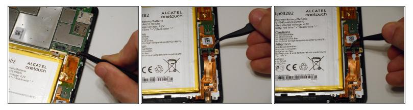
• We now need to remove 3 ZIF connectors, all located in the bottom right quadrant. The order they are disconnected doesn't matter.
