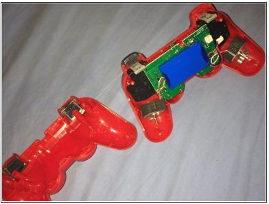
After you unscrewed all five screws in the back, next you're going to have to gently pull both of the controller sides apart and it will come straight off.
