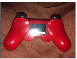
• First step you would have to do would be to unscrew five screws from the back of the controller.
